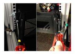
If the cable connectors had been mounted from the front side of ICEyslot the PC into the bottom most mounting rails of the rack and fix it using screws. Note: that the screws should go into 6 cm extenders. Also make sure that the rear mounting rails are positioned correctly before inserting the PC.
