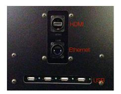
On the left and right side of the ICEySupport are terminals to connect external PC peripherals. On each side there are: 1 HDMI connector for an LCD screen, 1 Ethernet RJ45 connector for network access of the Control PC, 4 USB connectors for USB peripherals like mouse and keyboard.
