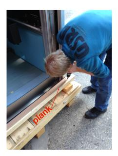
Remove the wooden planks securing the test chamber on the pallet base as shown on the left.
