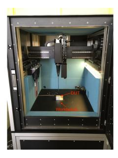
The ICEy Test Chamber contains a platform made from laminated glass. This platform is called DUT Workbench. That is where the DUT can be placed. The glass platform has a thickness of 10 cm and is backed with an RF absorber.
