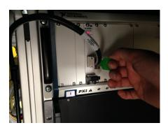
Fix the PXI inside the rack and connect the PXIe extension cable (from the Control PC) on the front side of the PXI chassis as shown.
