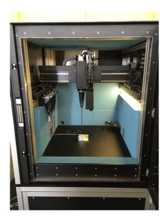
The positioning system is a Gantrytype system. With two x-stage, one y-stage, one z-stage and one roll stage to roll the probes around their axis. The camera system is suspended on the z-axis.
