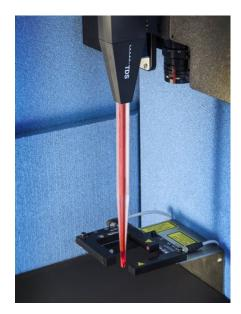
The probe tip location is reference in the fork light barriers. After ICEypicked up a probe its tip location is automatically referenced in the fork light barriers. During the reference also the repeatability of the light-barrier location is validated. The ICEy will warn the user if the repeatability is worse than 0.1 mm. A probe referencing can also be forced by the user from the ICEy GUI.
