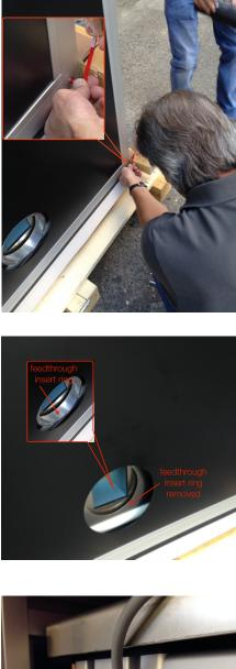
Remove the 4 grub screws at either corner of the decorative housing, securing it to the aluminium base of the ICEy Test Chamber as shown on the left using an Allen key.
