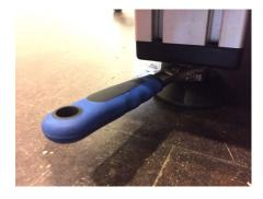
The support rack contains 4 adjustable feed. The feed can be adjusted and secured using a 19 mm wrench.
