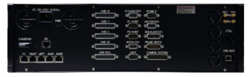
Figure 4.5: Connector allocation of the ICEy Interface Electronics (IE-ICEy).
