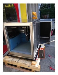
Lift the decorative housing (with 3 persons) sufficiently such that it is released from the locking pins shown on the left. Make sure not to lift the housing much further as it might otherwise not be possible to reverse with it. After lifting the housing from the locking pins, reverse with it and put it aside for later re-installation.
