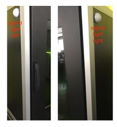
There is a signal light on either side of the chamber, indicating the system status to the user:
