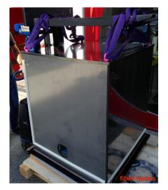
Install the lifting hooks on the top of the test chamber, if not installed yet. Use a forklift or a crane and appropriate lifting gear rated for the mass of the system to lift the ICEy Test Chamber off the pallet base of the transportation box. While doing so, make sure that none of the fiberoptics extending from below the Test Chamber rear, right connector terminal is damaged when lifting and moving the system.
