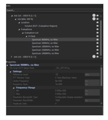
Figure 20.1: Scan job with multiple frequency domain scans and the signal generator control script selected as Pre Scan DUT Setup Hook.
