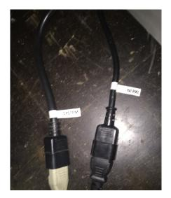
From the rear bottom of the equipment rack extend two power inlet cables, one for the PXI chassis and one for the rest of the system. These cables are IEC C14 types and can be easily customised with location specific IEC C13 power cords.
