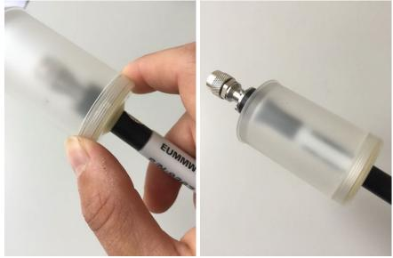
Align the notch and pin of the probe and DAE4ICEy connectors and carefully mate the probe connector with the DAE4ICEy connector. Make sure the probe body is straight and fasten the retainer nut carefully (not too tight). In the end screw on the probe cup and make sure the rubber seam is uniformely pointing upwards around the probe. Remove the protective cover before putting the probe inside the ICEy probe repository.
