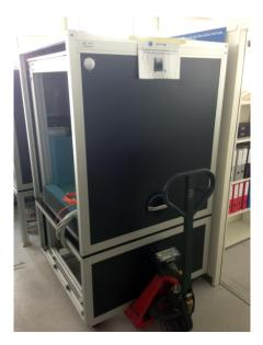
Use the pallet jack to move the entire ICEy to its destination. At the installation site use the adjustable feet to level the system and put it in place by lowering the pallet jack.
