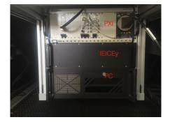
The ICEy rack drawer contain 3 19inch devices, the PXI Chassis with the Vector Signal Analyser, the IE-ICEy Interface Electronics and the Control PC.
