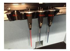
ICE y can hold up to four probes in its repository. The parking slots are numbered as indicated from the front to the rear side of the chamber.
