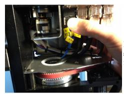
Reconnect the fiber optic connector saver at the top of the z-axis terminal.
