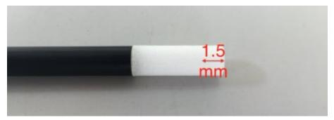
The sensors of the EUmmW probe are centred in the probe tip. The tipto-sensor centre distance is 1.5 mm.
