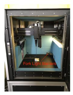
The fork light barriers are located the in the rear right corner of the system. The light barriers are suspended at a hight of 9 cm above the chamber floor. In this way DUT with a very large surface area can be placed also below the light barriers.
