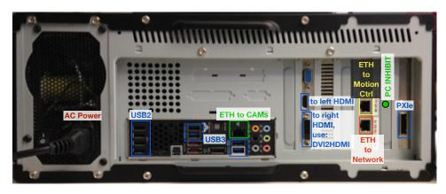
Figure 5.1: Connector allocation of the ICEy Control PC.
