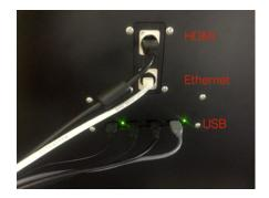
On either side of the rack there are 1 HDMI, 1 Ethernet, and 4 USB ports for connecting peripheral devices (mouse, keyboard, LCD) to the control PC.
