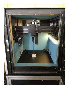
The ICE y Test Chamber is located on top of the equipment rack. It is a fully RF shielded chamber with a door that opens to the right side. Inside the test chamber the positioning system which perfors scanning is located. A LED light strip is located on the right side the probe repository holding up to 4 probes on the left side. Feedthroughs are available on the left and right sides as well as in the rear left corner.
