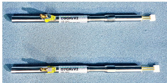
Figure 1.1: Two of the four dipoles (i.e., D7GHzV2 and the D9GHzV2) used for system performance checks in the frequency range between 6 – 10 GHz
