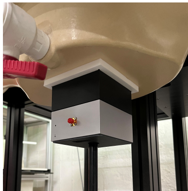
Figure 1.3: P6500V2 positioned under the Flat phantom for SAR/APD system check
